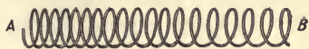
FIG. 133.—Waves Transmitted by a Spring. The Individual Turns Move back and forth while the Waves Progress along the Spring.
